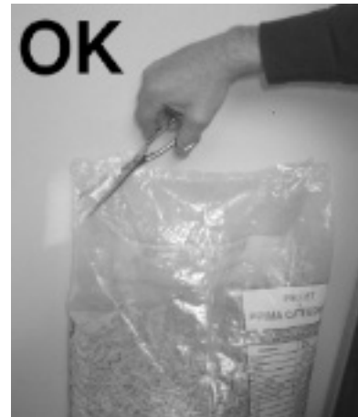
Fig. 14 - Right opening of the pellets bag
