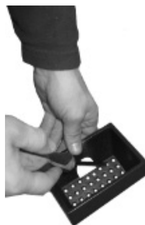
Fig. 38 - Burning pot cleaning
